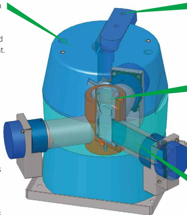
Measurement chamber with high reflective opaque paint maximises light collection.
